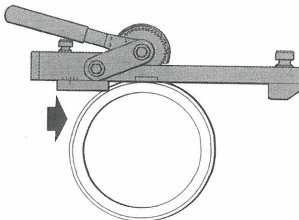
Drop the drive wheel down to grip the bead.
